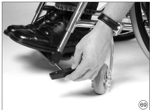
**Adjusting the Angle of the Footplate Avantgarde Ti 8.9 and Ti Ultra**
