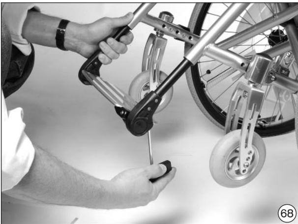
**Adjusting the Angle of the Footplate Avantgarde T, VR and XXL 2**
