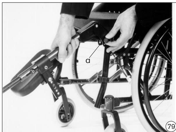
**Angle Adjustment of the Elevating Avantgarde VR and XXL 2 Footrests**
