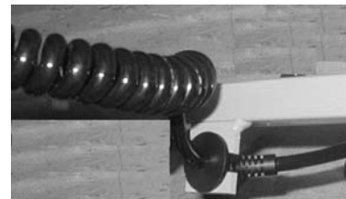
Fig. 15: traction relief network cable
