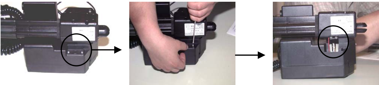
Fig. 25: exchanging the backup battery
